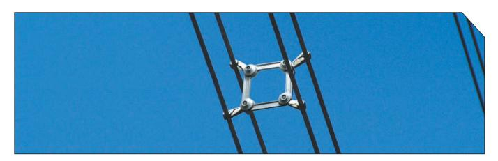
Spacer Dampers are recommended for multi-conductor bundles with industry standard spacing. The Spacer Damper is designed to withstand the forces and movements caused by transient conditions such as short circuit, differential icing, and wind loading without either causing damage to the sub conductors or sustaining damage themselves. The design accommodates both longitudinal movement of the sub conductors, vertical sag differences, as well as compressive and tensile forces.
